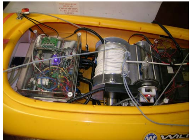
Fig. 2. SCOUT equipped with autonomous winch (center). The main vehicle computer is visible on the left.
