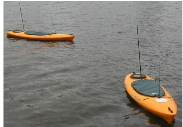
Fig. 10. Two kayak-based autonomous surface craft for used for in-field experiments. Each had access to GPS and shared their current position and trajectory with the other.
