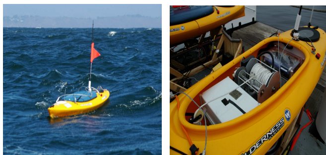
Fig. 4. The kayak-based autonomous surface craft. These lightweight and portable platforms are not only suitable proxies for the much larger autonomous underwater vehicles but also show the suitability of autonomous surface craft for oceanographic sampling. The left photo shows an autonomous kayak on station in Monterey Bay while the right photo shows details of the autonomously controlled winch used to raise and lower the Seabird Electronics SBE 49 FastCAT CTD sensor.
