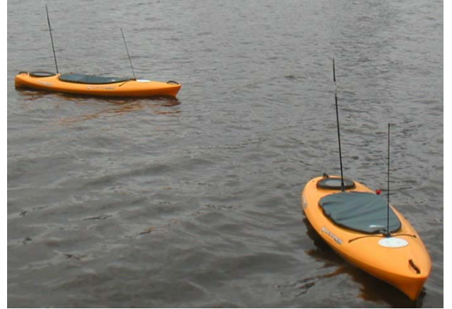
Fig. 10. Two kayak-based autonomous surface craft for used for in-field experiments. Each had access to GPS and shared their current position and trajectory with the other.
