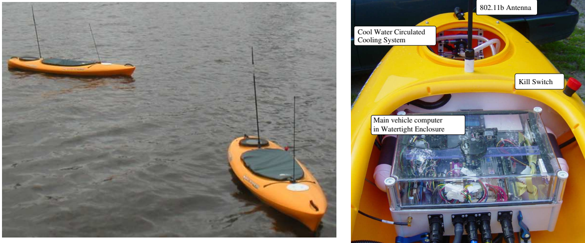
Figure 10: Two kayak-based autonomous surface craft for used for in-field experiments. Each had access to GPS and shared their current position and trajectory with the other.
